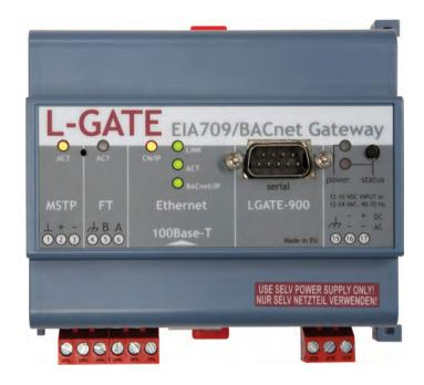
The BACnet gateway (EC660) is a CEA-709/BACnet gateway which maps CEA-709 network variables (NVs) to standard BACnet server objects. When ordered with this part code EC660, the LonWorks to BACnet address mapping is pre-loaded and ready for use with the Eaton Easicheck board.
